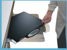
To rotate the tray hold the receptor and lightly pull clockwise.
